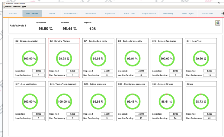
Picture 1: REAL TIME SPC PLATFORM – REAL TIME YIELD AT MULTIPLE STATIONS AT ONE AUTOMATIC ASSEMBLY CELL
